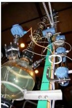
9 Rosemount<sup>®</sup> wireless pressure transmitters and 7 Rosemount wireless temperature transmitters have been installed
