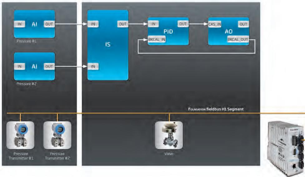
Figure 2: The CiF's PID function block uses process values to calculate valve input.
