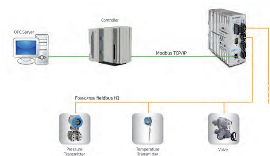
Figure 1: Remote field devices are connected to the central controller via Modbus/TCP and remote gateways.
